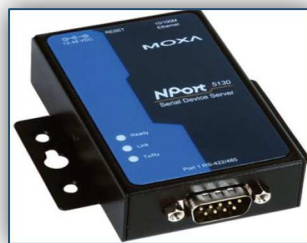
Figure 39. Ethernet to RS-485 converter module.
